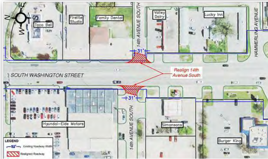
FIGURE 7.7 – 14th Avenue South Realignment
