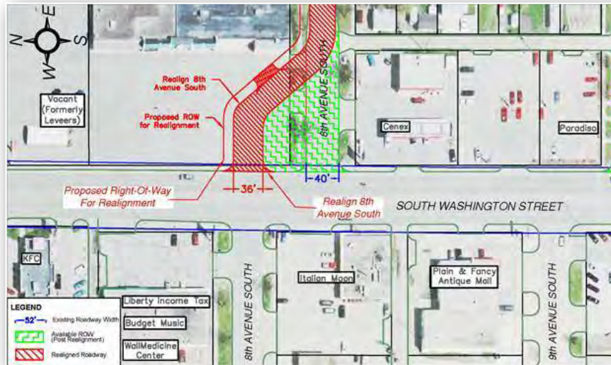
FIGURE 7.9 – 8th Avenue South Realignment
