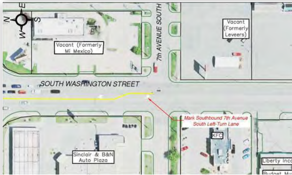
FIGURE 7.10 – Marked Southbound 7th Avenue South Left-Turn Lane
