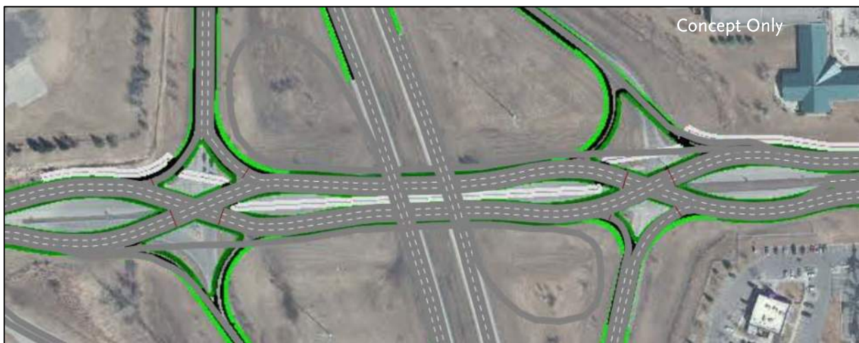
Figure 7-23: Diverging Diamond Partial Cloverleaf Alternative (Existing Interstate Access Scenario)
