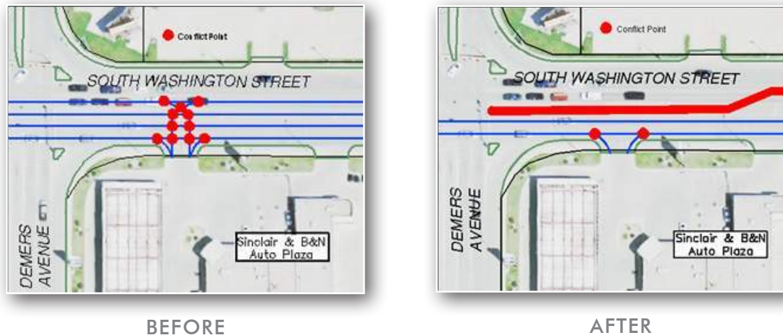
FIGURE 7.3 – Example of Conflict Elimination Through Median Control
