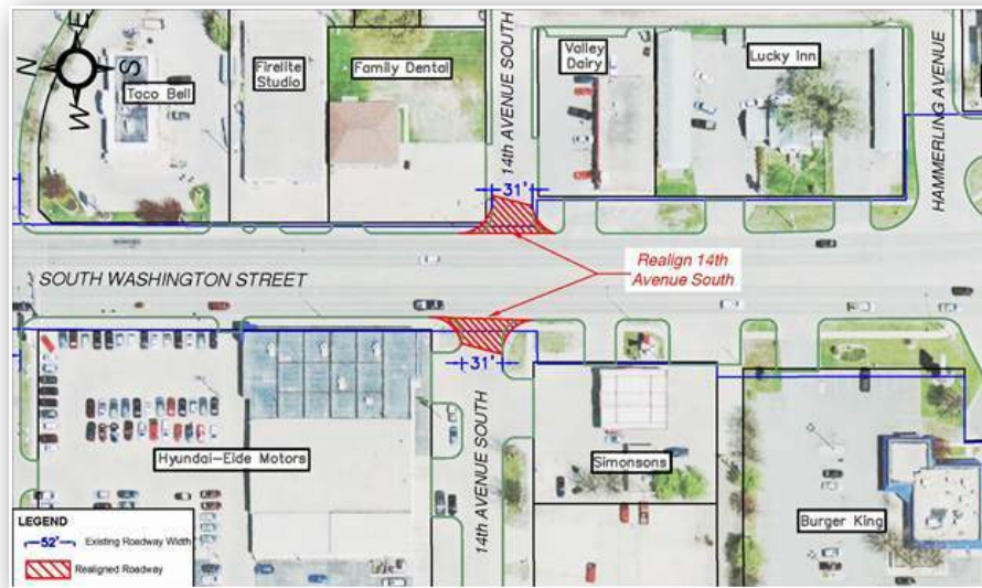
FIGURE 7.7 – 14th Avenue South Realignment
