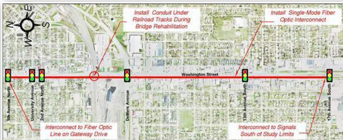
FIGURE 7.4 – Corridor-Wide Traffic Signal and Video Monitoring Interconnection
