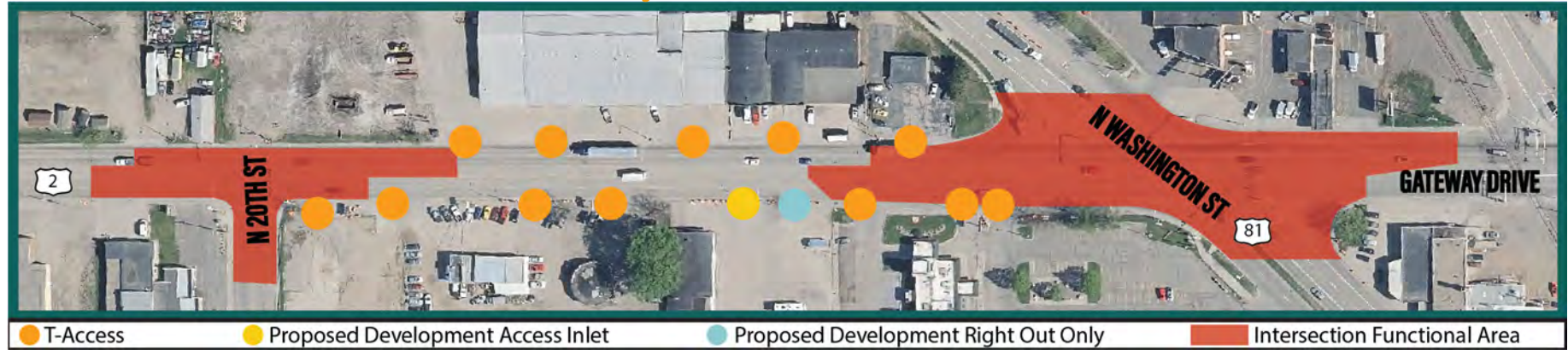
Figure 21: Intersection Functional Area
