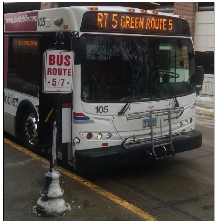
Figure 7-16: Bicycle Rack on Fixed Route Bus
